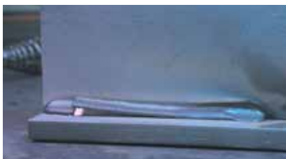
Self peeling slag from a weld made with Arcos E309L.
